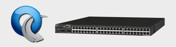
Forwarding elements that implement packet-processing functionality efficiently in hardware
